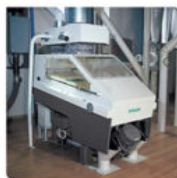
MTSD destoner for efficient separation of stones and pebbles
